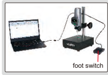
data transmitted to Excel without software
